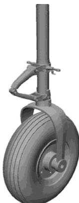
extended. (Prevents rudder pedals from moving the nose wheel prior to touch down) The point here is, don't be tempted to over inflate the strut to make up for the winter days ahead cause you might just defeat your steering capability on the first warm day. That could make for some excitement on the taxiway on your visit to a fall fly in. (in front of all your friends).
